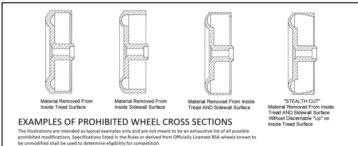
Figure 3 Examples of Prohibited Internal Modifications
