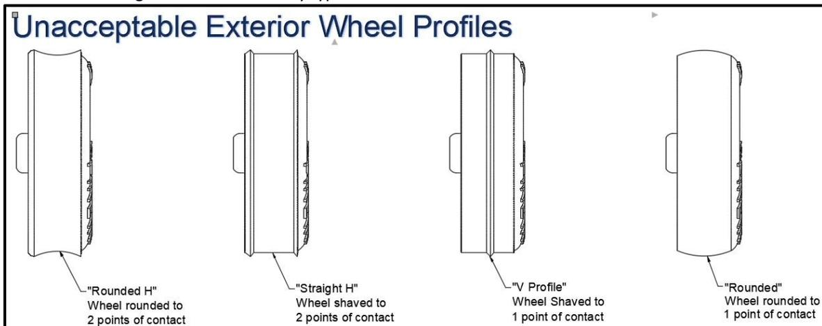
Figure 2 Unacceptable Exterior Wheel Profile
