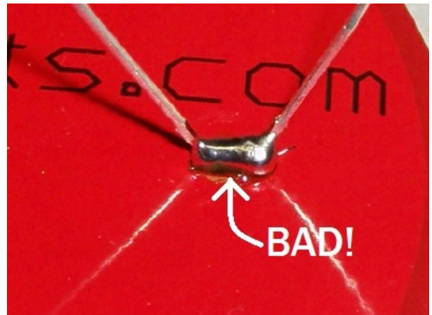
A bridge between the two leads of the LED. Current will flow through the bridge, and not the LED, thus the LED will not light up. Fortunately, this is easy to fix.
