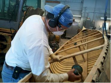
Sanding between coats gives the inside of the canoe a beautiful shine. Every inch of exposed wood must receive the same level of care, ensuring that the canoe will be around for years to come. Lastly the outside of the canoe will be coated in fiberglass and painted, before being reassembled.
