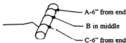
Tie at points A-B-C with 2' of rope left on C
