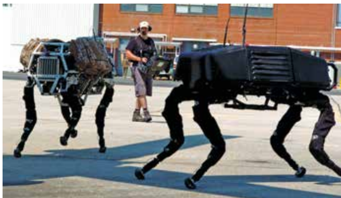
The BigDog “pack mule,” a four-legged robot, is designed to help carry supplies for U.S. military troops.
