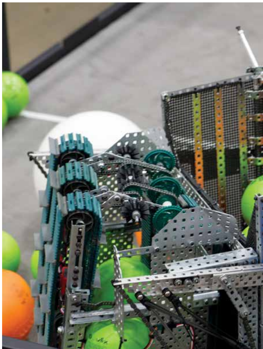
A robot's power system connects to axles, gears, wheels, or other forms of locomotion through the chassis. In many robot designs, the motion and chassis subsystems are tightly integrated.
