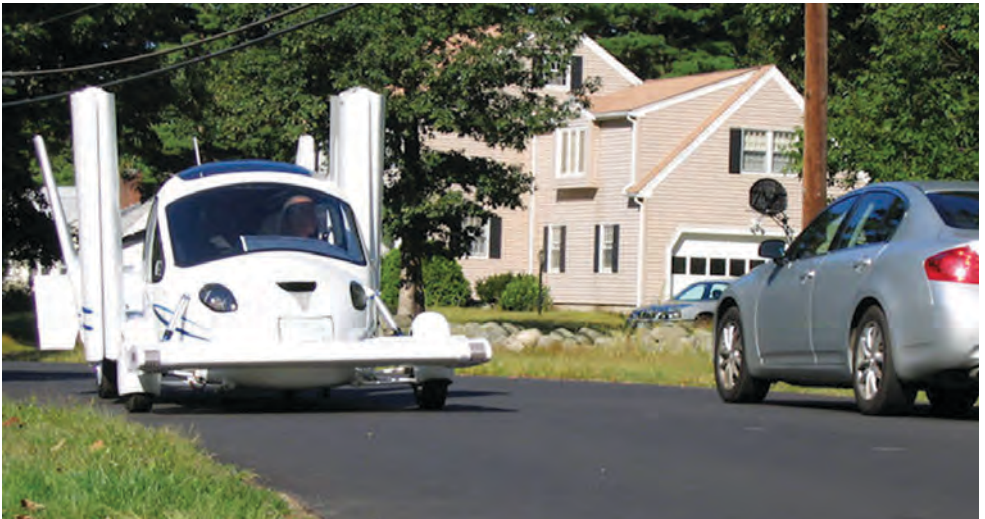
The Transition roadable aircraft is a plane that can fold its wings and be driven along the road like a car.
