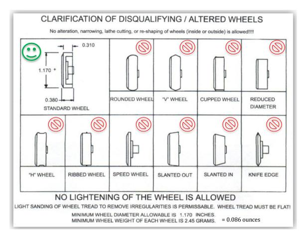
Please note: There are after-market modified wheels available that have been LIGHTENED. This is usually done by turning the wheels on a lathe and removing material from the inside of the wheel. These wheels are **NOT** allowed and can be EASILY RECOGNIZED at inspection. Cars with third party manufactured or modified wheels will not be permitted to race or will be disqualified from trophy placement.
