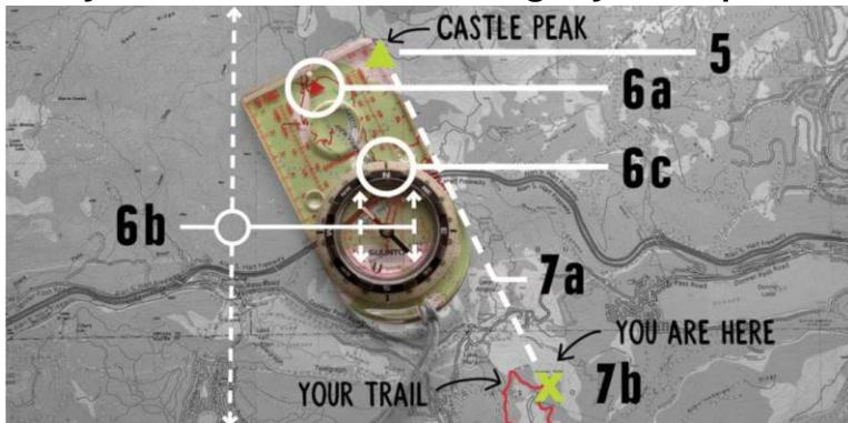
Lay your compass on the map and align one corner of the straight edge with the landmark.
