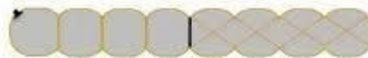
Chambered "air" mattress: (L) open tubes, (R) baffled air chambers - lengthwise or across width.
