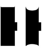
Shaped for Only Two Points of contact **left** to reduce friction (commonly called H profile**l**e)
