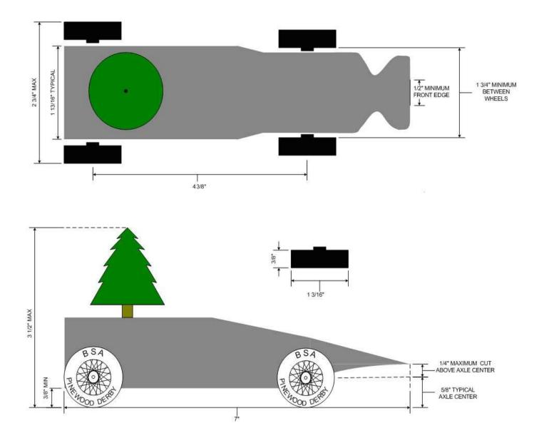
Sample layout of a car with dimensional guidance
