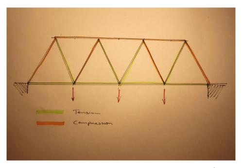
Bars are either under tension or compression by highlighting the components under tension/compression in different colors (see diagram above).
