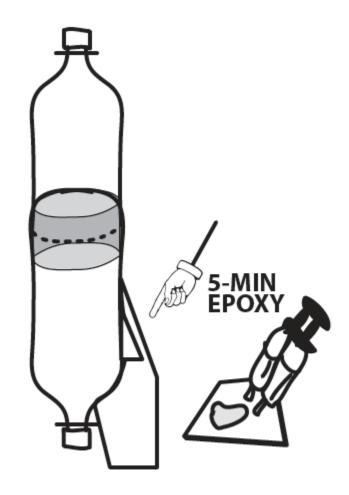
This is the added step for extra support. Glob out another dab of Epoxy and glue your triangle to the bottle and the fin. Glue the Supports on each side of each fin. Wait approx 10-15 minutes to be sure Epoxy has set.
