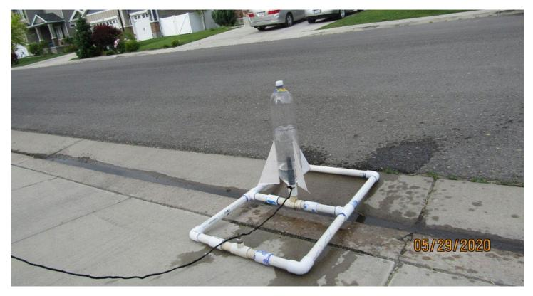
Add enough water to the pressure chamber so that is 1/3 full. Put it on your rocket launcher (there are more than one, 2 liter bottle rocket launcher Instructables, on this web site) and add +/- 80 psi air pressure,
