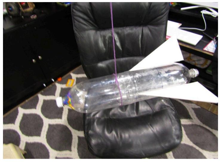
How take the string and find the center of mass of the whole rocket. Do it the same way you did when you found the center of pressure. Having the center of pressure forward of the nozzle and having the center of mass and quite a ways forward from the center of pressure will prevent the rocket from tumbling and flipping (these unwanted movements are called pitch and yaw).
