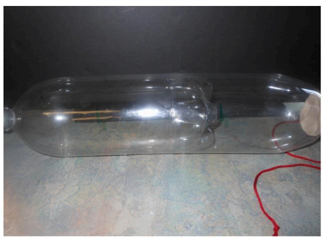
Slide the cut end of the nose cone over the bottle of the gas chamber. Do not tape this piece on yet.
