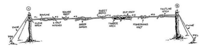
\*Lashings/Knots used: clove hitch, bowline, two-half hitches, square knot, sheet bend, timber hitch, slip knot, fisherman's knot, taut-line hitch, sheep shank.
