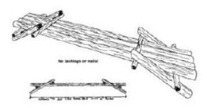
Solution: The Bridge must be made by interlocking the logs so that friction locks it together. Logs placed on the ground like a log cabin will not score, see diagram. Catapult Competition:
