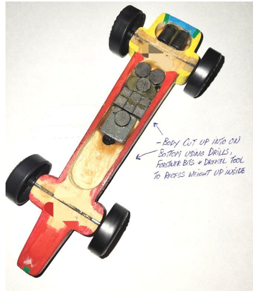
Figure 2 - Underside of Car (Legal)
