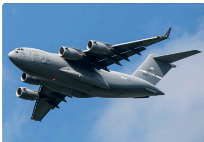
C-17 Globemaster II The newest heavy lift transport in the US military. It can haul 85 tons– an Abrams tank, 10 armored Humvees, or 100 paratroopers and all their gear. It can
